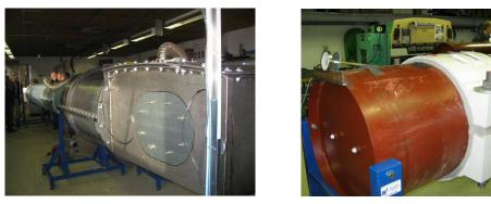
Figure 13 Full scale testing of sealing, left saddle and shroud, right cable band and transition at band
