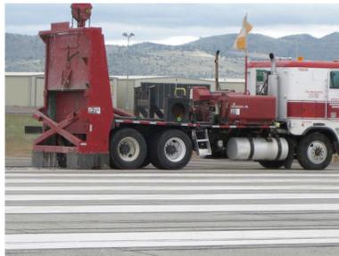
Six-ton guillotine hammer used for breaking concrete
