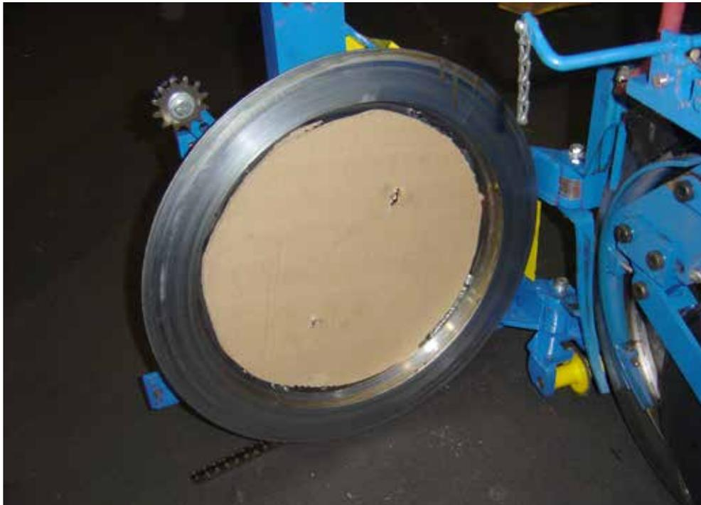
*Figure 18 Place Cardboard Cutouts Inside Compression Blade*
