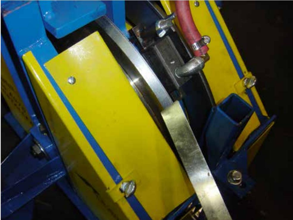
*Figure 16 Cleaning Compression Blades with a Putty Knife*
