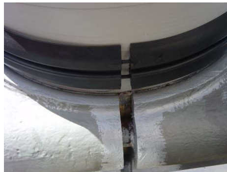
FIGURE 12 WEDGE GAP AND PLASTIC BARBS
