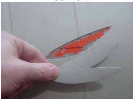
FIGURE 34 PUNCTURE REQUIRING CUT PROCEDURE
