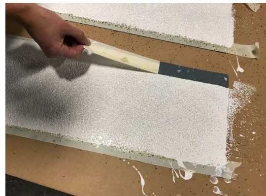
FIGURE 27 MASKING TAPE BEING REMOVED DIRECTLY AFTER TOP COAT APPLICATION
