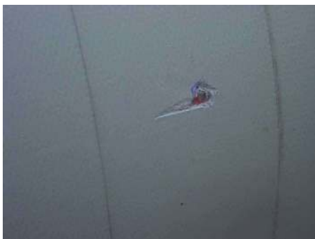
FIGURE 34 PUNCTURE REQUIRING CUT PROCEDURE
