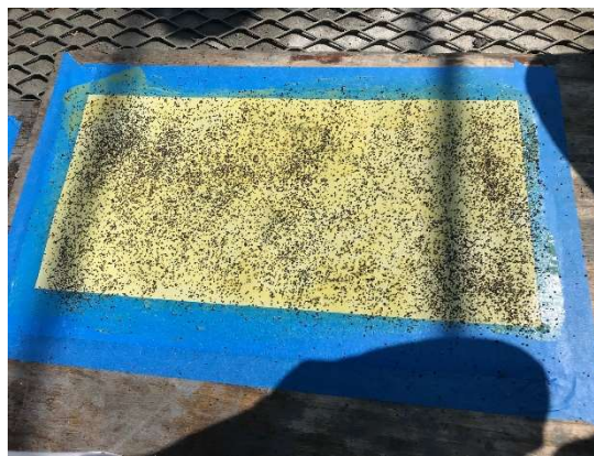
FIGURE 25 CORRECT GRIT APPLICATION
