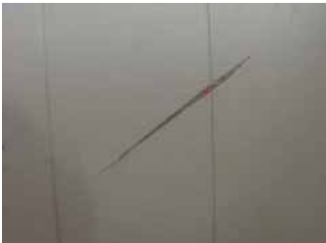
Figure 32 Cut Less Than 75mm Long
