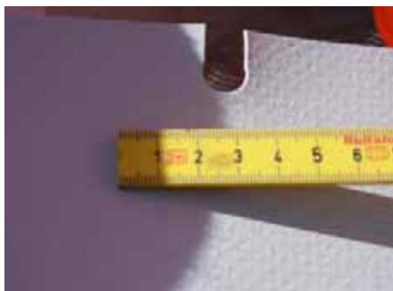
Figure 24 10mm Wide By 15mm Long Slot For the Wedge Gap on the Upper Cable Band
